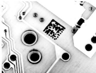
Figure 24 - Data Matrix Code Directly Marked on PCB Surface by Using Laser Etching Technology
